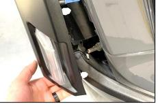
7. Free the bottom trim piece for the grill by pulling directly away from the vehicle.
